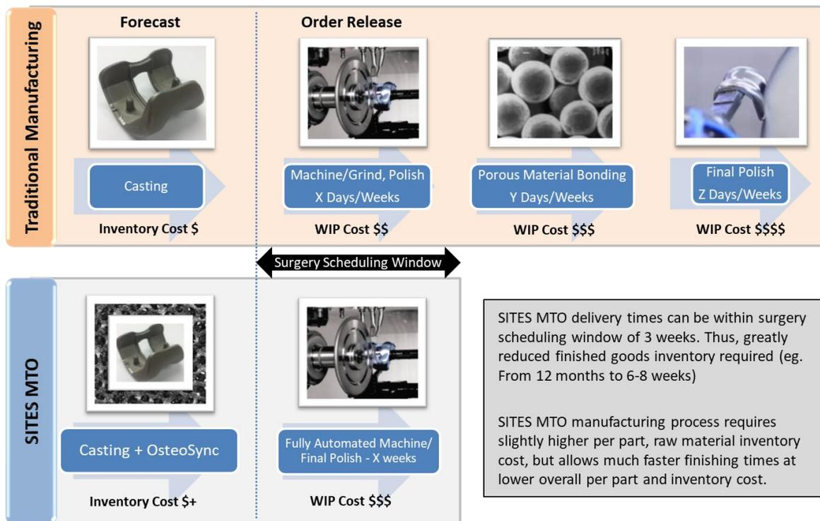
The SITES Medical CoCr Stabilization and *OsteoSync Ti* technologies are already in commercial use. The MTO process requires size inputs which are readily obtainable from systems that many OEM's already use such as patient specific instruments or robotic platforms – each of these takes in calibrated images (radiograph, CT, MRI) that can be used for implant size determination and they facilitate implant placement with a minimum of instrumentation and often in single-use, disposable form.
